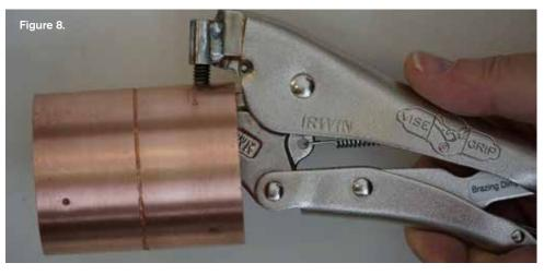
One also could modify the fitting so the tube does not slide all the way in by putting a limit stop inside the fitting. That is easily done using a product such as the Brazing Dimpler® or something similar shown in Figure 8. This tool forms a dimple on the outside of the fitting which protrudes on the inside of the fitting 1/2 in., or so back from the fitting end.
