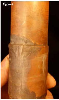
The technician should be able to show the thickness of the fitting, the tube and, at the brazed or soldered joint, the sum of the fitting thickness plus the tube thickness. The technician can then scan joints and map out filled and unfilled zones as shown in Figure 5. I have successfully used this arrangement on sockets down to 1/2-in. tube size joints.
