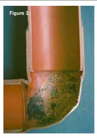
Figure 2 shows a cross-section of a brazed joint that only is partially filled; the unfilled crevice is a notch that intensifies the stress at the interface between the members and if there is any vibration, that notch will propagate and eventually result in a leak.
