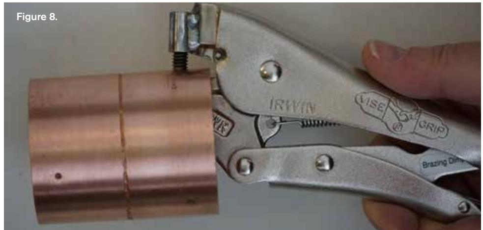
One also could modify the fitting so the tube does not slide all the way in by putting a limit stop inside the fitting. That is easily done using a product such as the Brazing Dimpler® or something similar shown in Figure 8. This tool forms a dimple on the outside of the fitting which protrudes on the inside of the fitting 1/2 in., or so back from the fitting end.
