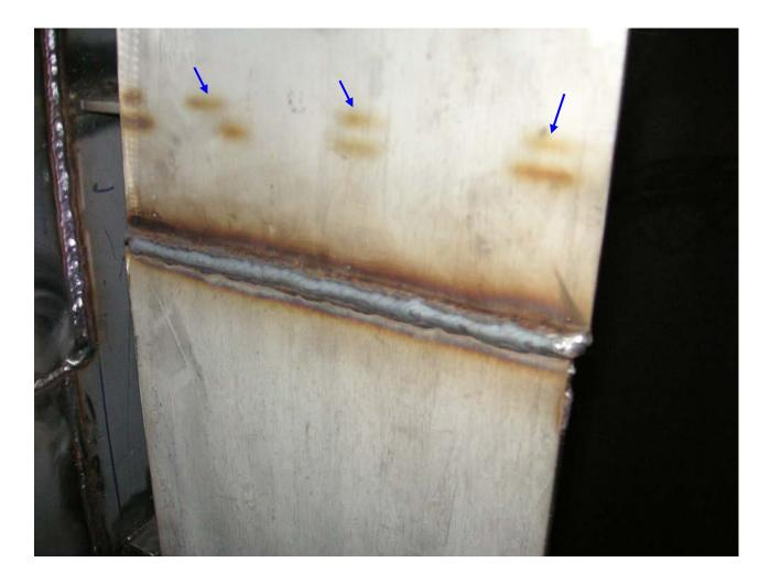
The photograph shows rust on a stainless steel plate.
