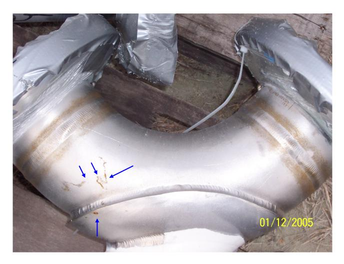
The photograph shows rust on a stainless steel pipe spool piece.
