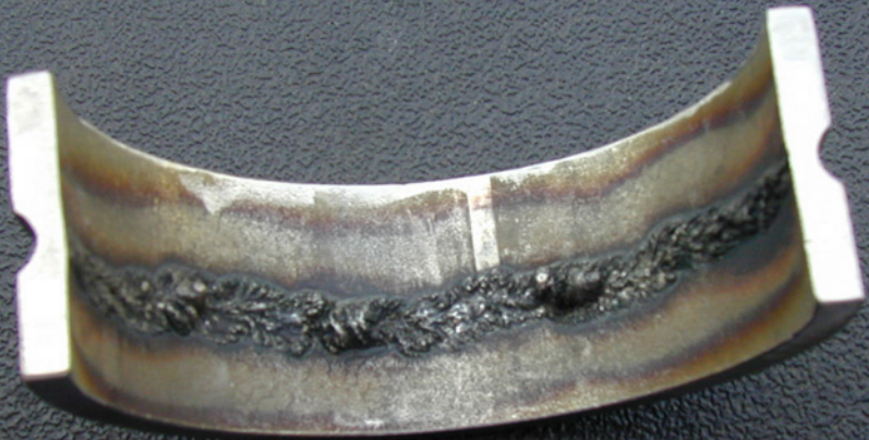
Typical weld in stainless steel made without backing gas
