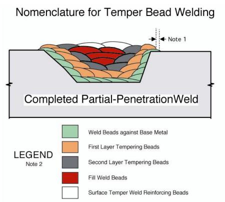
Note 1: This is the distance from the edge of the surface temper beads to the toe of the weld. Note 2: Beads near the finished surface may be both tempering beads and surface temper reinforcing beads
